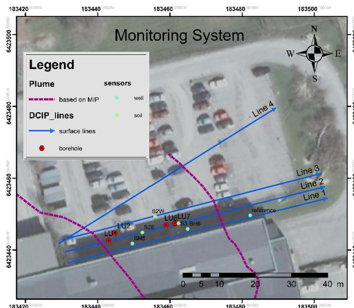
Figure 3. Monitoring system installations.
