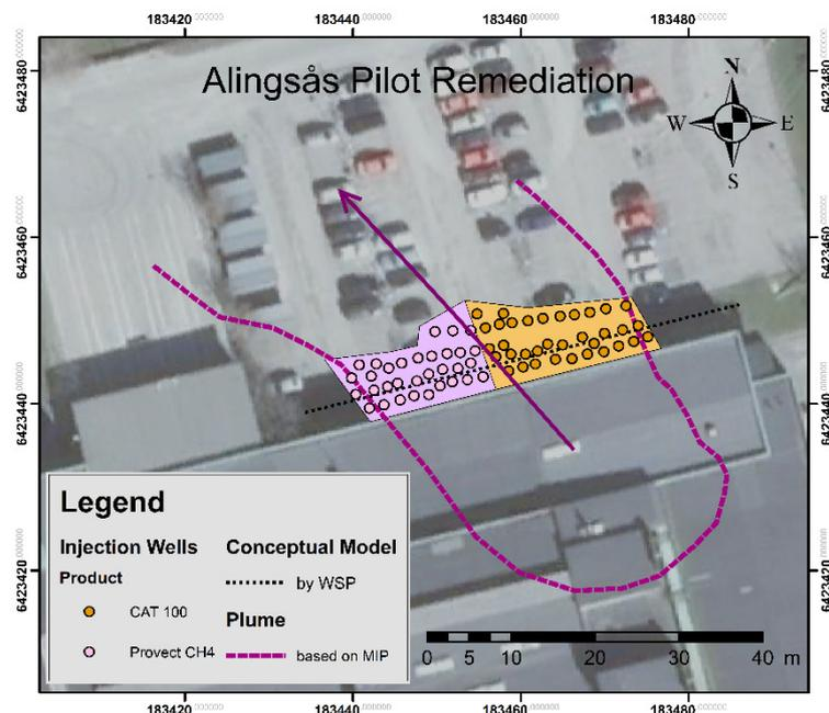
Figure 1. Alingsås contamination plume and remediation plan.
