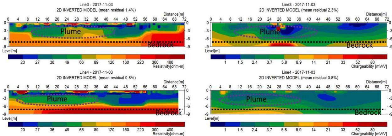
Figure 3. Results from the baseline measured with the autonomous system. Resistivity results (left) and chargeability results (right).
