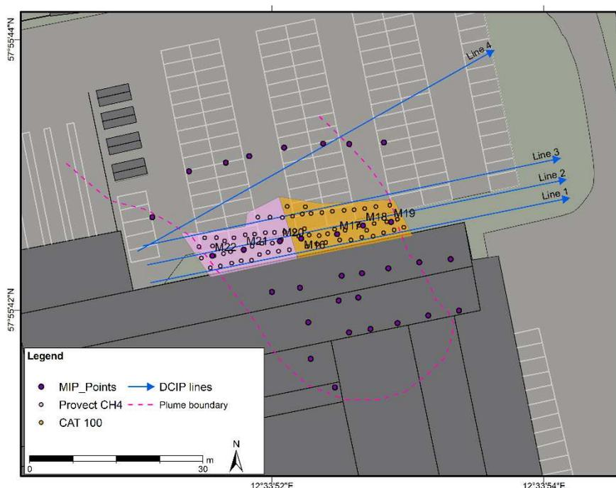
Figure 1. Overview map showing location of contaminant plume, DCIP lines, MIP soundings and pilot in-situ bioremediation injection points.
