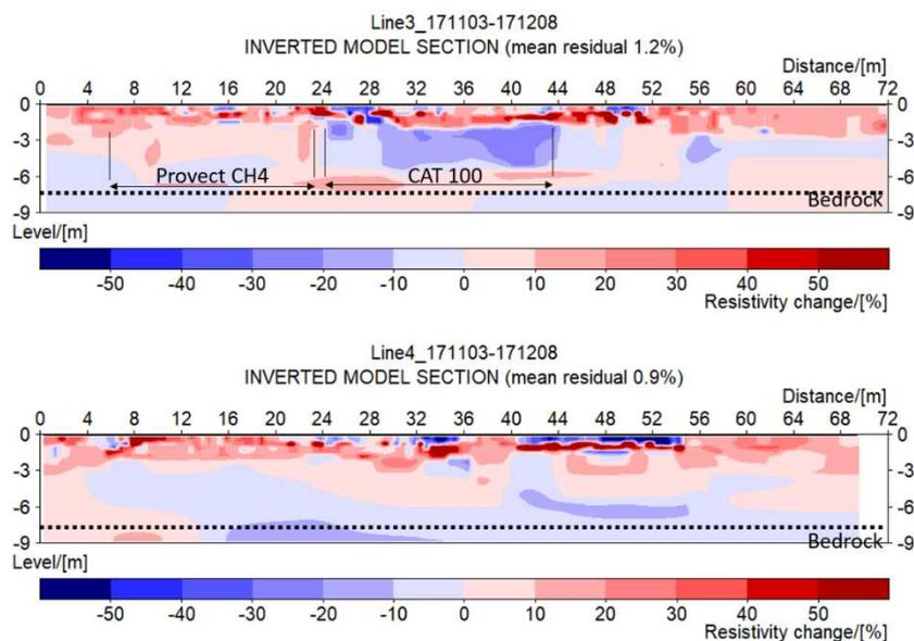
Figure 4. Time-lapse results showing the effects right after the injection. The areas where the injection took place are marked in Line 3 and are projected into Line 4.
