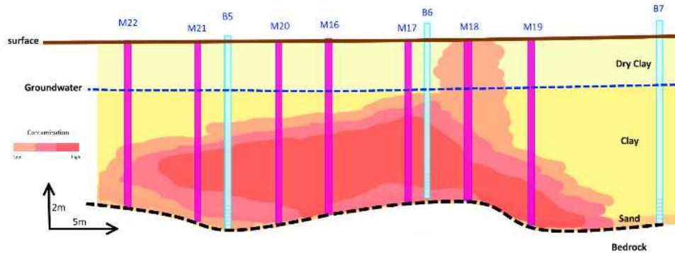
Figure 2. Simplified geological model based on the MIP sounding (provided by WSP).
