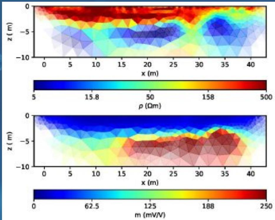
Figure 3. Geophysical inversion results showing the resistivity  $\rho$  (top) and chargeability  $m$  (bottom) distribution of the subsurface in several meters depth along a measurement profile. Different colour zones can be seen, which can be interpreted as specific underground structure.
